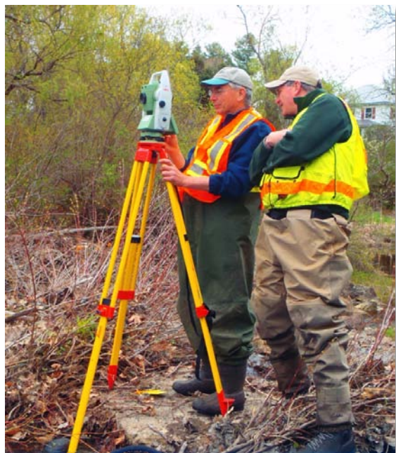
Elevation measurements were collected with a Total Station to help quantify the changes expected from dam removal.
