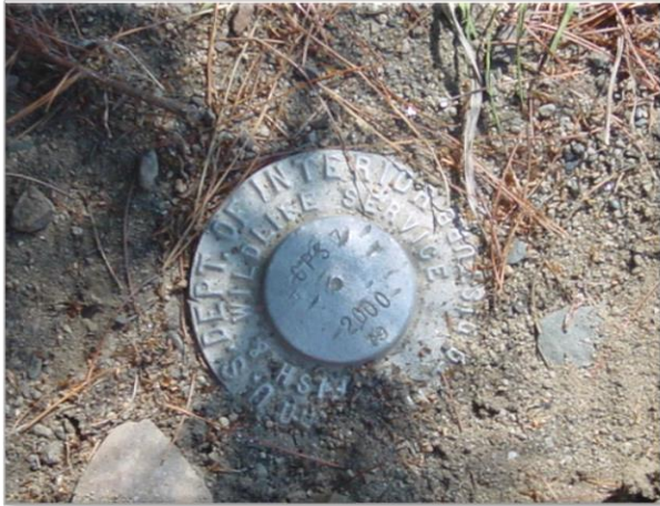
Establishing vertical control in Wheeler Refuge allows elevation measurements to be collected within the National Spatial Reference System used by NOAA to maintain tide stations and forecast flood elevations.
